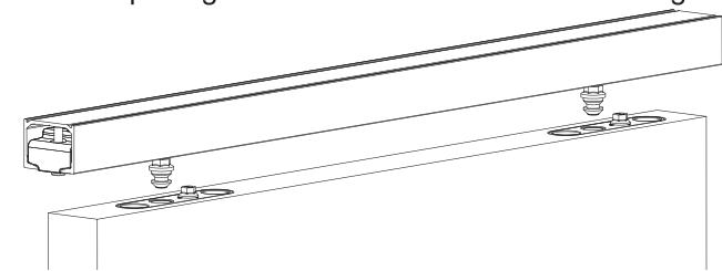
(b) Use the spanner to turn the locking lever 90 degrees clockwise so the arrow points to the lock symbol.
