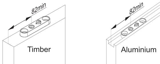
(b) Route 12mm recessed slot (timber only) and pre-drill pilot holes for 10G screws.
