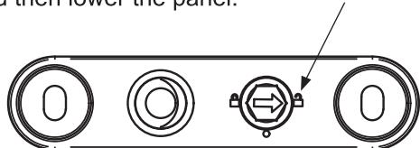
(b) Make sure to turn the locking lever to installation position after the panel is removed.
