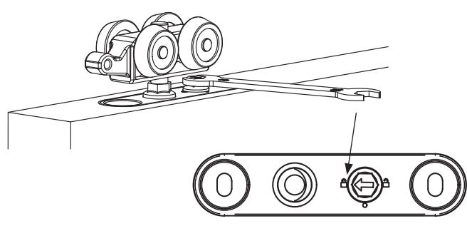
(c) Adjust the height using the spanner provided. Clockwise rotation will lower the panel, and anti-clockwise will raise the panel.
